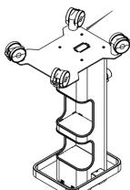
• Take out the bottom plate and install it on the pillar of the Cart. Use a screwdriver to tighten the bottom screw.
